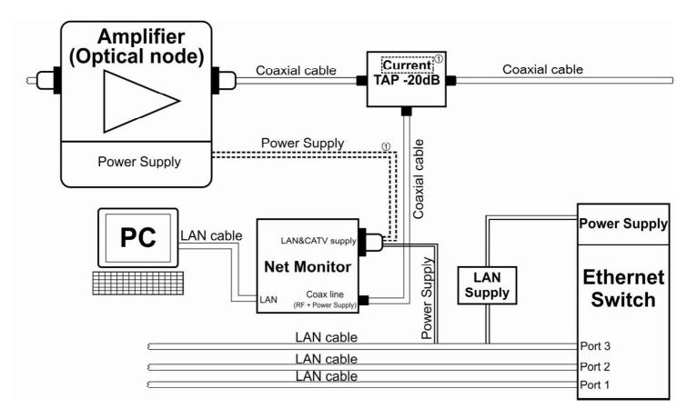
1 When power is not available on the coaxial line the voltage can be measured directly from the power supply. In this case there is no need to use current Tap.
